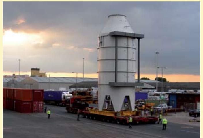
18m tall, 250 ton Coil, being moved locally within Hull on a 10-axle 4-file [double width] trailer Photo courtesy of GCS Johnson Ltd
