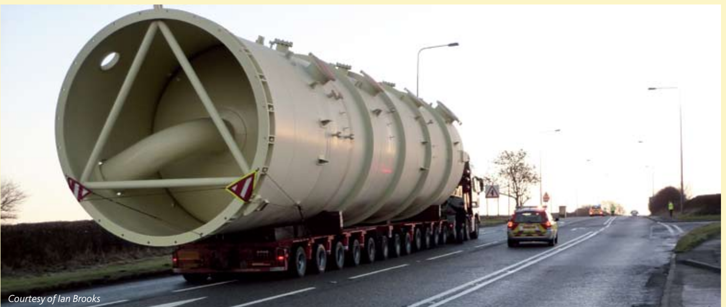
Photo courtesy of Cadzow Heavy Haulage Ltd 80 tonne ducting being moved at a power station
