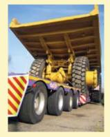
The key to load security is appreciating that any load has its own dynamic independent of the vehicle on which or in which it is being carried. A common fallacy is the heavier the load the less the need to restrain it. Nothing could be further from the truth. The heavier the load the greater the potential kinetic energy it exerts. If the vehicle stops or changes direction its load will continue to exert a dynamic force in the direction
